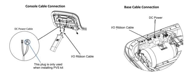
Connect the main interface ribbon cable and DC power cable to corresponding connectors on the console. At the treadmill base connect the main interface ribbon cable and DC power cable to the corresponding MCB connectors.
