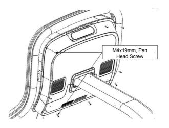
Secure rear console bottom shroud to console in the correct position with six M4 x 0.7 x 19mm, Pan Head Screws, then secure console top rear shroud to console in correct position with eight M4 x 0.7 x 19mm, Pan Head Screws, tighten all screws securely.
