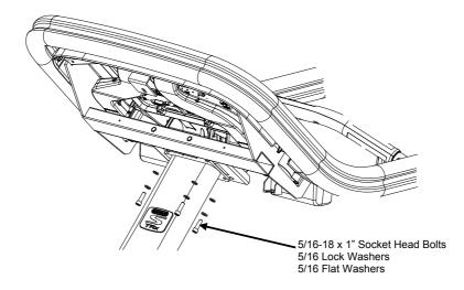
Locate and position the display console on the neck, taking care not to pinch the display cable between the neck and the console. Once the console is properly positioned, secure the console to the neck using four  $5/16"-18 \ge 1.0"$  socket head bolts, 5/16 lock washers, and 5/16" flat washers. Install all four bolts then tighten securely.
