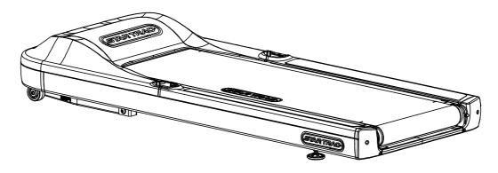
Remove all packaging material so the base assembly is sitting on the shipping crate platform. With a helper, lift the base assembly from the shipping crate platform, and place it in the location where it will be used. Be sure the selected location is level, and close to a power outlet. Remove the motor shroud for installation of the handrails.
