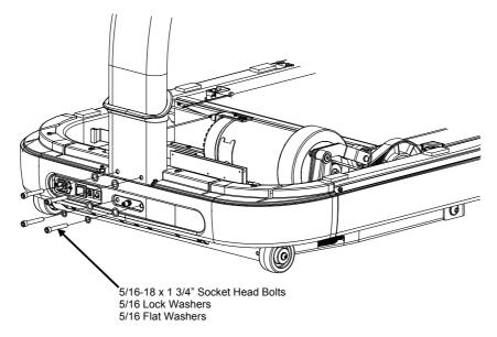
Locate the neck assembly (Qty. 1) and neck grommet (Qty 1) with console cables pre-installed inside. Remove packing material and slide the neck grommet over the neck. Position the neck in place on the motor end of the base assembly and secure with four  $5/16"-18 \ge 2.0"$  socket head bolts, 5/16 lock washers, and 5/16" flat washers. Install all four bolts then tighten securely.
