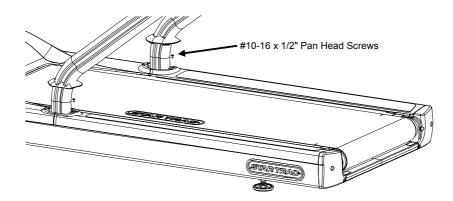
Remove the paper layer of the adhesive tape located on the back of side tread plates, now install the tread into position on the base assembly with one  $\#10-16 \ge 1/2$ " tapping pan head screw.
