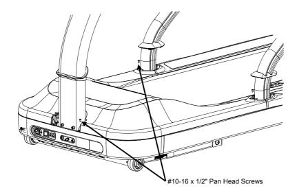
Remove the paper layer of the adhesive tape located on the back of the motor top cover, secure the front end of the cover to base assembly with two  $\#10-16 \ge 1/2$ " tapping pan head screws, then secure the back end of cover to base assembly with two  $\#10-16 \ge 1/2$ " tapping pan head screws.
