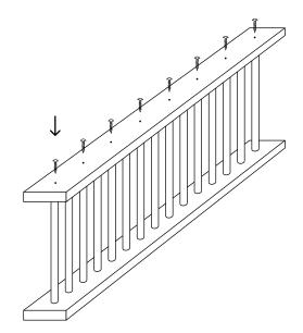
The remaining 4 dowels and screws are used to mount the ladder to the wall. Any steps of this manual where hammer is required, we highly recommended to use spacer (wood, plastic, hard rubber etc.) to balance the force and prevent destroying a gantla materials.
